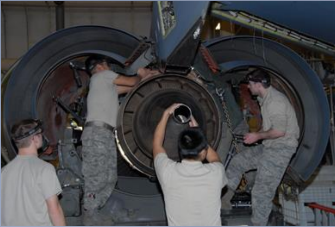
Maintenance Airmen from the 168th Maintenance Group had the opportunity to replace an engine from one of the KC-135R Stratotankers assigned to the Interior-Alaska unit. The entire process takes several days and involves Airmen from multiple shops within the maintenance group. (U.S. Air National Guard photo by Airman 1st Class Mae S. Olson)
