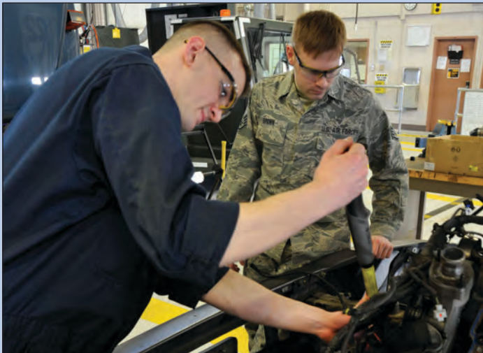
Top Airman. While reconstructing an engine, Senior Airman Shaun Hageman, a 168th Air Refueling Wing Vehicle Maintenance Flight vehicle mechanic, checks the torque of parts of an engine in February 2015. Hageman won several awards in 2015, including Alaska Air National Guard Airman of the Year. Photo: Master Sgt. Cornelius Mingo, 168th Air Refueling Wing
