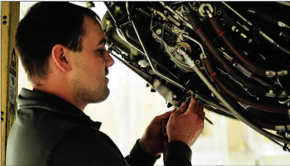
Engine Maintenance. Staff Sergeant Josh Thompson, 168th Air Refueling Wing aircraft engine mechanic, takes measurements on the engine of one of nine 168th Air Refueling Wing KC-135 tankers to ensure that the plane is ready for flight. Photo: First Lieutenant Bernie Kale, DMVA Public Affairs
