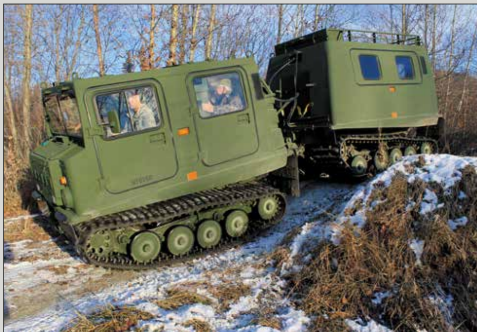
Go Anywhere. Alaska National Guardsmen and mechanics from the Red River Army Depot near Texarkana, Texas, test drive two M973 Small Unit Support Vehicles on and around Joint Base Elmendorf-Richardson, Alaska, in November 2014. SUSVs are fully-tracked, all-terrain, amphibious vehicles designed to support platoon-sized units in arctic and mountainous conditions. The Alaska Guard received the two SUSVs from the Red River Army Depot in November as part of an initiative to maintain its arctic vehicle capability. Photo: 1st Sgt. Charles Hooper, Alaska Army National Guard
